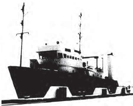
RV Ranger vehicle used for testing a precise time transfer receiver (TTR) in mobile mode. (Oaks-1995, p. 402)
