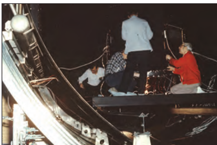
Setting the satellite in NRL's large temperature-vacuum test chamber. (NRL Photo)
