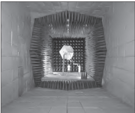
Anechoic chamber, in which NTS-2 was tested. (NRL Photo)
