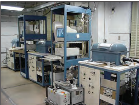
A selection of PCEF equipment, from top: Reference Environmental Chamber, Large Thermal Vacuum Chamber, Three Axis Helmholtz Coil, and Life Test. (NRL Photos)
