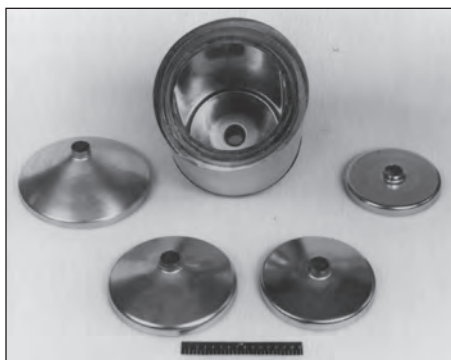
Photograph of a nested set of maser magnetic shields and their end caps. (Wolf-1978, p. 141)
