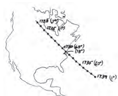
TIMATION II satellite ground track for 16 November 1971 pass. (Easton-1971, p. 65)
