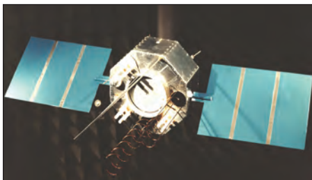
Satellite testing in NRL's anechoic chamber. (NRL Photo)
