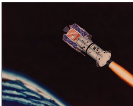
The NTS-2 satellite with solar paddles folded during launch. (Walker-1979, p. 5)
