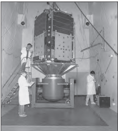
Acoustic test facility. (NRL Photo)
