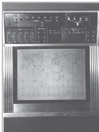
SPACECORE satellite map display for Space Surveillance System. Past, present, or future position of all known and selected satellites is updated by the minute. (NRL Photo)
