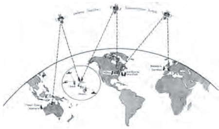
Schematic proposing global time transfer with the Defense Satellite Communication System (DSCS). (Murray-1970, p. 78)
