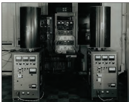
Hydrogen masers at the Naval Research Laboratory. Hydrogen Maser I on the right has operated for 6 years as the NRL standard. (Phillips-1970, p. 329)
