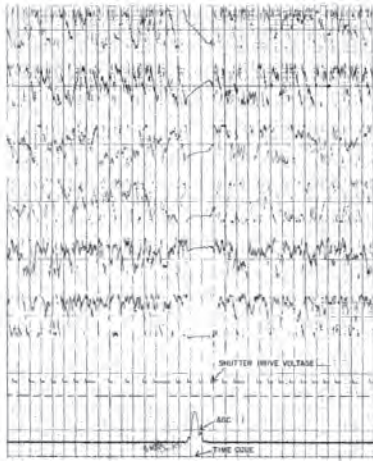
Sample of the recorded data from which the zenith angle of the satellite is determined. (Hayden, NRL5741-1962, p. 5)
