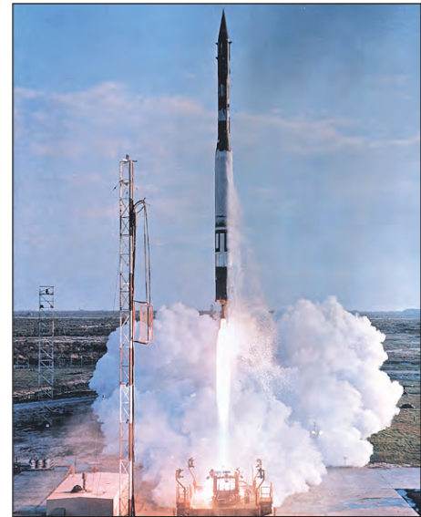
Vanguard launch, 17 March 1958. The third stage of the rocket used solid propellant to thrust the second American satellite into orbit. (NRL photo)
