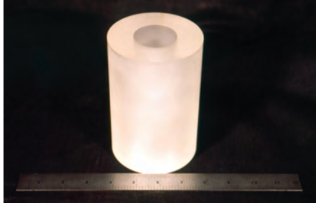
Sapphire maser cavity. (White-1980, p. 505)
