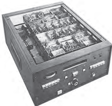
400 Megahertz time dissemination receiver. (Easton-1971, p. 59)
