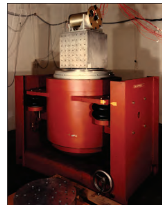
Nested magnetic shields for hydrogen maser undergoing pre-flight shake testing at NRL. (NRL Photo)
